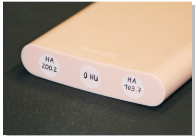
QRM-Bone in the Bone Calibration Phantom
