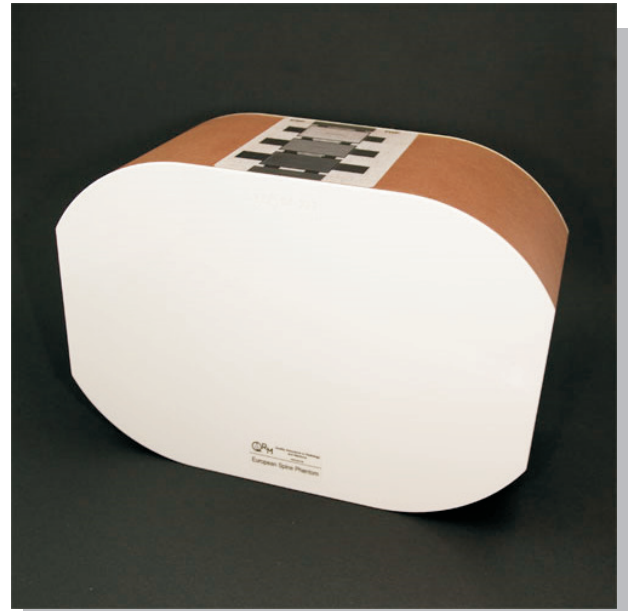
Resin based water-equivalent phantom body approximately oval shape but with flattened sides for ease of positioning.
