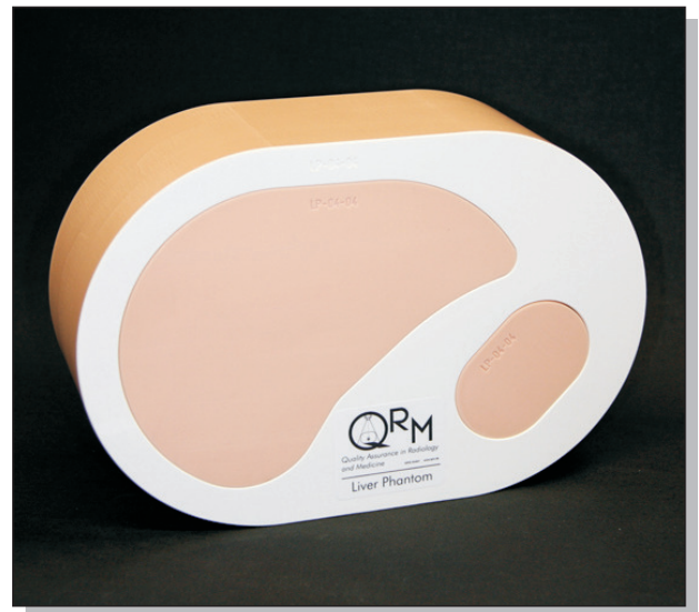
QRM-Liver-Phantom with exchangeable liver insert
