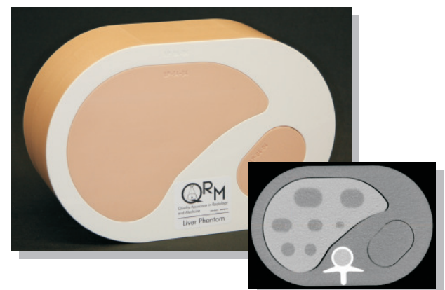
Example for a tissue equivalent liver phantom with nodules
