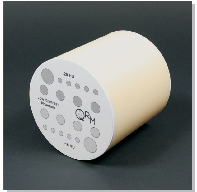
2DL with different contrast cylinders of -10 HU and -20 HU!
