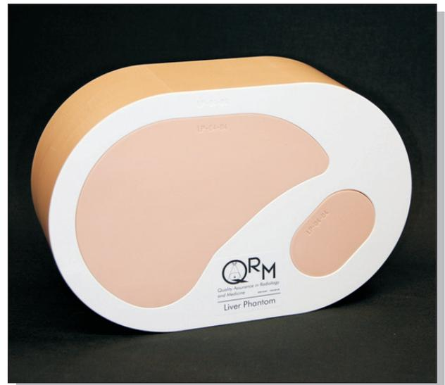
QRM-Liver-Phantom with exchangeable liver insert
