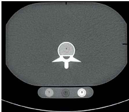
Figure 12: Cross-calibration example (ESP with BDC Phantom)
