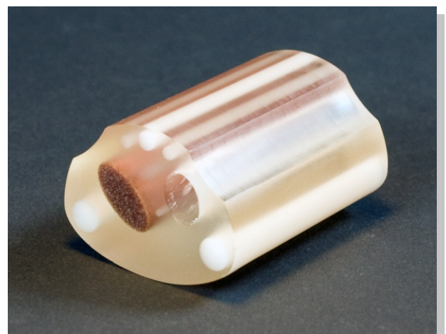
Bone equivalent inserts in the QRM-MicroCT Mouse Phantom
