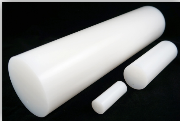
Micro-PET NEMA-NU4 Scatter Phantoms Mouse, Rat and Monkey Size
