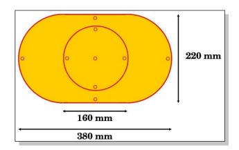
Schematic view of the phantom
