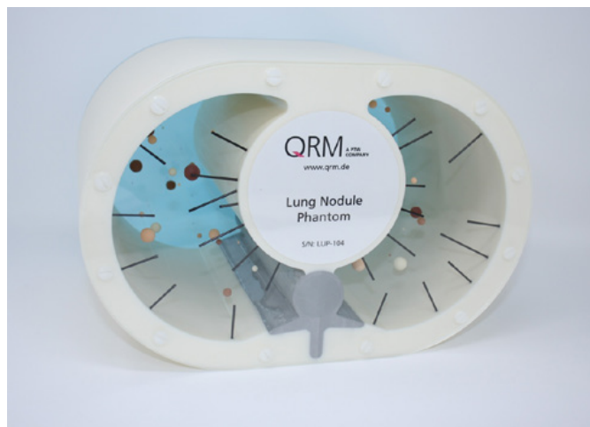
Figure 1. QRM Lung Nodule Phantom for realistic quality assurance in low-dose CT lung cancer screening.
